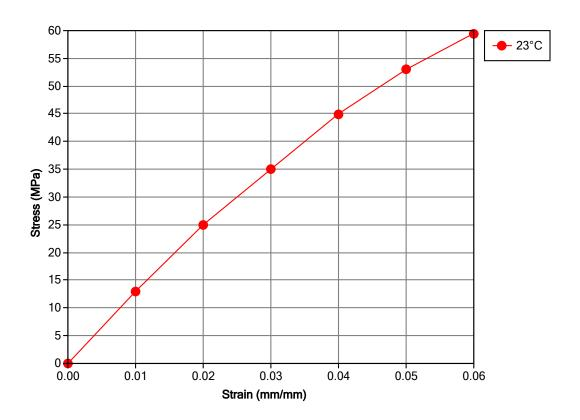
Secant Modulus vs. Strain (ISO 11403-1)
