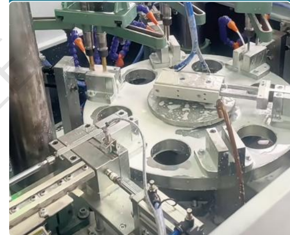
Fully automatic drilling and tapping integrated processing
