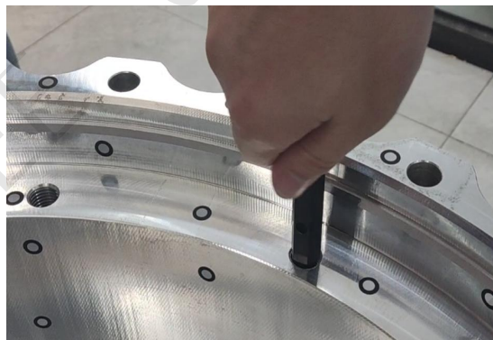
5: All threads go through gauge inspection
